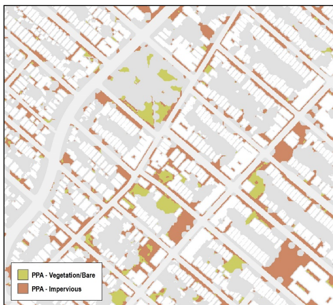
A Possible Planting Area (PPA) analysis was performed at a city-wide scale using the best data currently available. This image shows PPA area broken out by surface type - Impervious (e.g. parking lots, sidewalks) and Non-Impervious (e.g. grass, bare earth).
