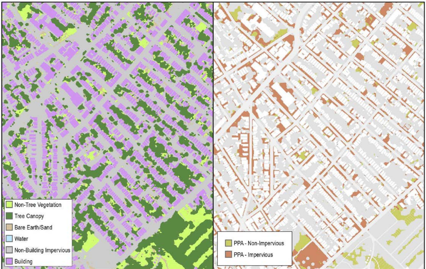
Figure 6 The map at left shows Urban Tree Canopy data for a part of Jersey City, New Jersey. The map at right shows the predicted Possible Planting Area for the same geographic area. Note that two types of Possible Planting Area are distinguished: Impervious (e.g. parking lots, sidewalks) and Non-Impervious (e.g. grass, bare earth).
